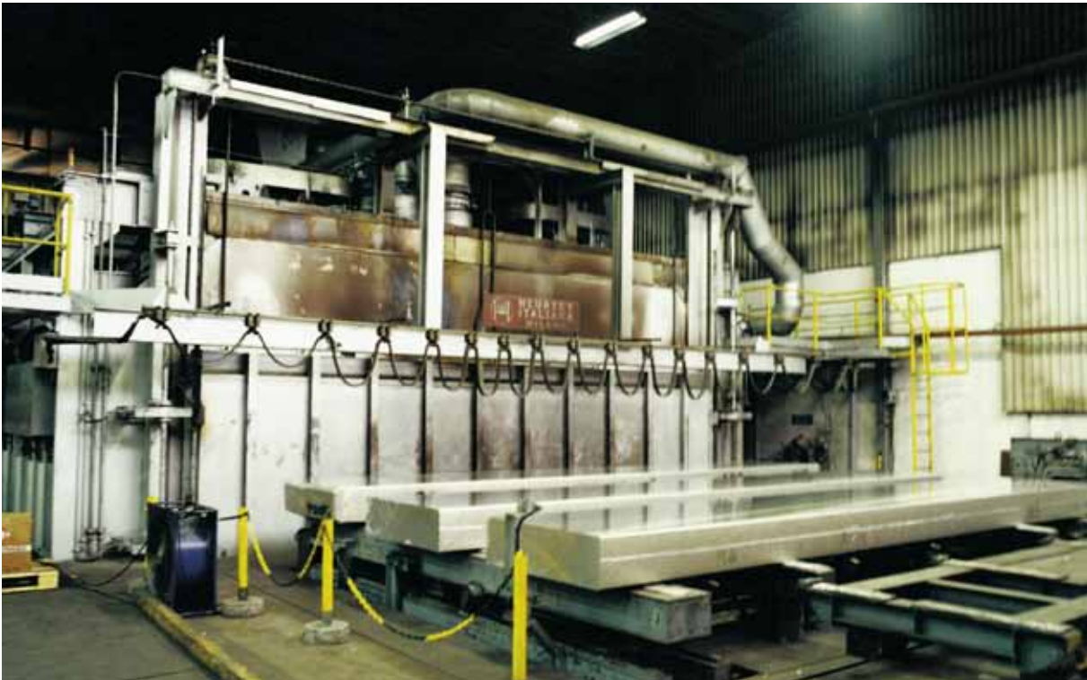
The pusher furnace at Hydro Aluminium Holmestrand, Norway. The 7-ton slabs are heated to 600°C (1110°F) before rolling by eight Kanthal heating cassettes, four on each sidewall.
