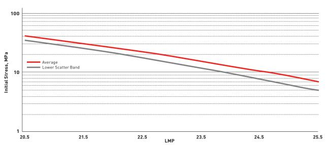
LMP = Larson Miller Parameter. LMP = T (15.0 + log tr )/1000. Where T: temperature [K] and tr: rupture time [h]. Lower Scatter Band represents 95% confidence level
